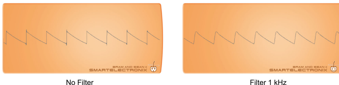
A low-pass filter rounds off the edges
